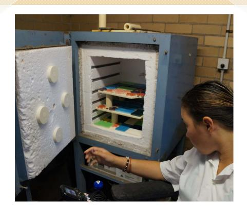
Opening the kiln after a glaze firing is so exciting. As long as no clear glaze touches the kiln surface, nothing should get stuck.
